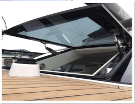
17MM LAMINATED TG - FLUSH WINDSCREEN - POWERED OPTION
