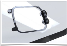
MOULDED TO HULL SURFACE PROFILE - INCLUDING INTEGRAL PORTLIGHT
